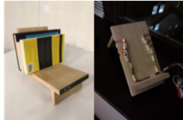
**Figure 1.** Top view of bookshelf (left), wiring and circuit view of bookshelf using conductive tape and alligator clips to connect to an Arduino (right).
